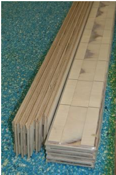
Backside of the Lumaflex panel – this side must be installed on the foam
