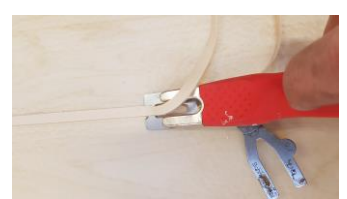
Second trim with a Mozart knife after cooling.
