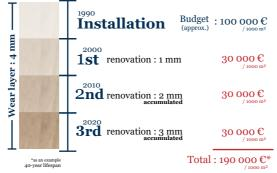
Renovation works are considerabily expensive since they include sanding, varnishing and retracing of lines.
